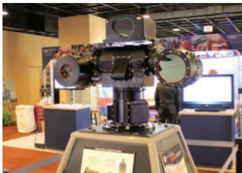
L-3 will provide MK20 shipboard electro-optical sights to help keep naval gunfire on target.
