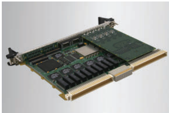
The VME-690 24-Port 6U VMEBus Gigabit Ethernet switch module from Curtiss-Wright provides a 35-watt, pin-compatible replacement for earlier designs while adding advanced data security features.
